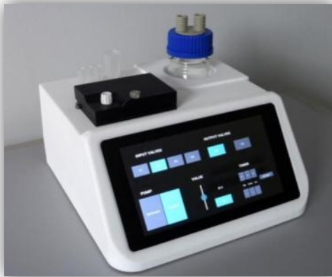
Integrated system (left) for detecting bio-compounds using disposable cartridges (right)
