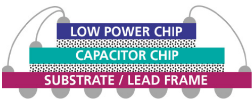
Non-volatile SRAM co-packed with ultrathin high density silicon caps as System in Package (SiP)
